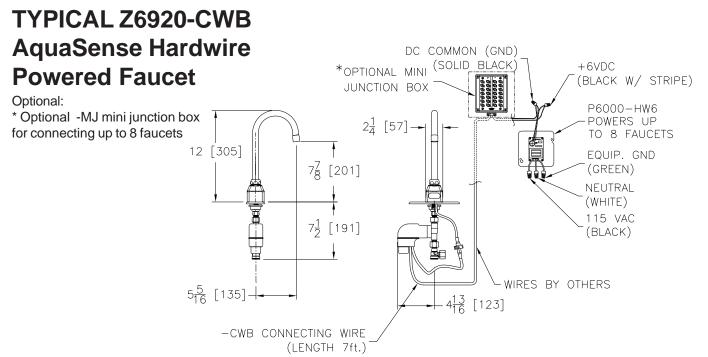
NOTE: MUST USE EITHER ZURN P6000-HW6 HARDWIRE POWER CONVERTER OR ZURN P6900-ACA PLUG-IN POWER CONVERTER TO ENSURE PROPER OPERATION. USING A POWER CONVERTER OTHER THAN ZURN MAY RESULT IN OPERATION MALFUNCTION OR UNIT FAILURE.
