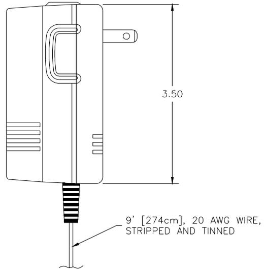
**ENGINEERING SPECIFICATION: ZURN P6000-PC6 AquaSense Multi-Unit Power Converter** - The AquaSense Multi-Unit Power Converter is designed to provide 6 VDC power for up to eight Zurn 6 VDC sensor flush valves. The unit is a 120 VAC plug-in style power converter with a 9' [273cm] 6 VDC output cord.
