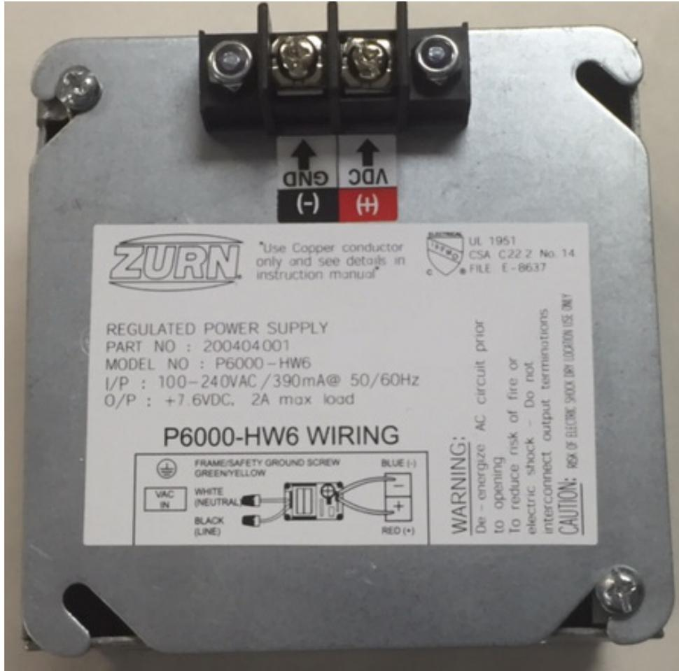
**P6000-HW6 (7.6VDC) Hardwired Power Converter for Flush Valves and Faucets**
