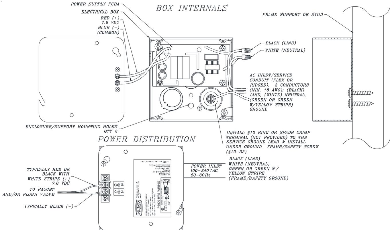
The internal (Line & Neutral) conductor terminations/connections, shall be implemented using UL approved screw terminals, wire nuts, insulated crimp splices, or soldered using hook & loop method with the solder joint(s) post insulated or as specified within the National Electrical Code (NEC) and/or superseding relevant local specified code(s).
