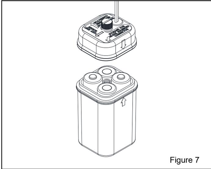
**⚠** Only use one battery type for installation. **DO NOT** mix and match Standard (Alkaline) and Long Life (Lithium) Batteries.
