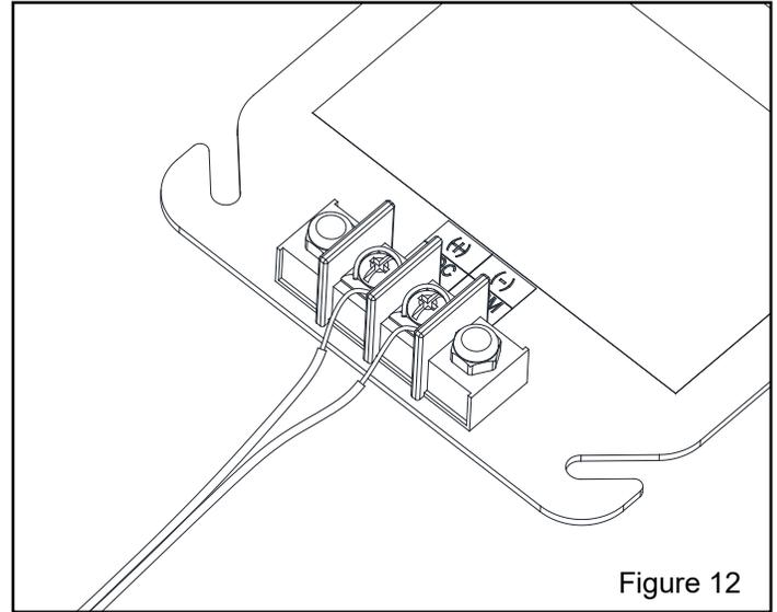
Optional Junction Box (recommended when three or more ZTR flush valves utilize one HW6)
