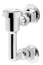
Engineering Specification: Zurn AquaSpec® Z80000-EVB Polished chrome-plated brass elevated atmospheric vacuum breaker assembly for concealed piping. Unit is provided with 3/8" [10mm] short swivel inlets providing adjustable centers from 2-7/8" [73mm] to 4-3/8" [111mm]. Unit conforms to ASSE 1001 and CSA B64.1.1.
