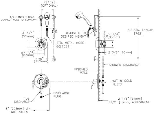
Note: All dimensions are for reference only. Do not use for pre-plumbing. Parts shown as hidden lines are supplied by others.
