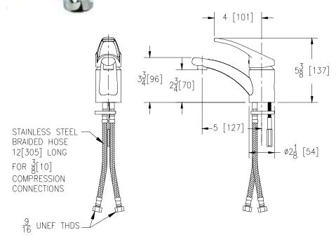
Zurn Lead Compliant\* "XL" products are a line of durable, high quality brass faucets and fixtures that are designed and manufactured to comply with state laws and local codes that mandate lead content levels. Zurn "XL" products are manufactured with \*not more than 0.25% lead content when used with respect to wetted surfaces of pipes and pipe fittings, plumbing fitting and fixtures: California Health & Safety Code § 116875; Vermont 9 VCA § 2470h
