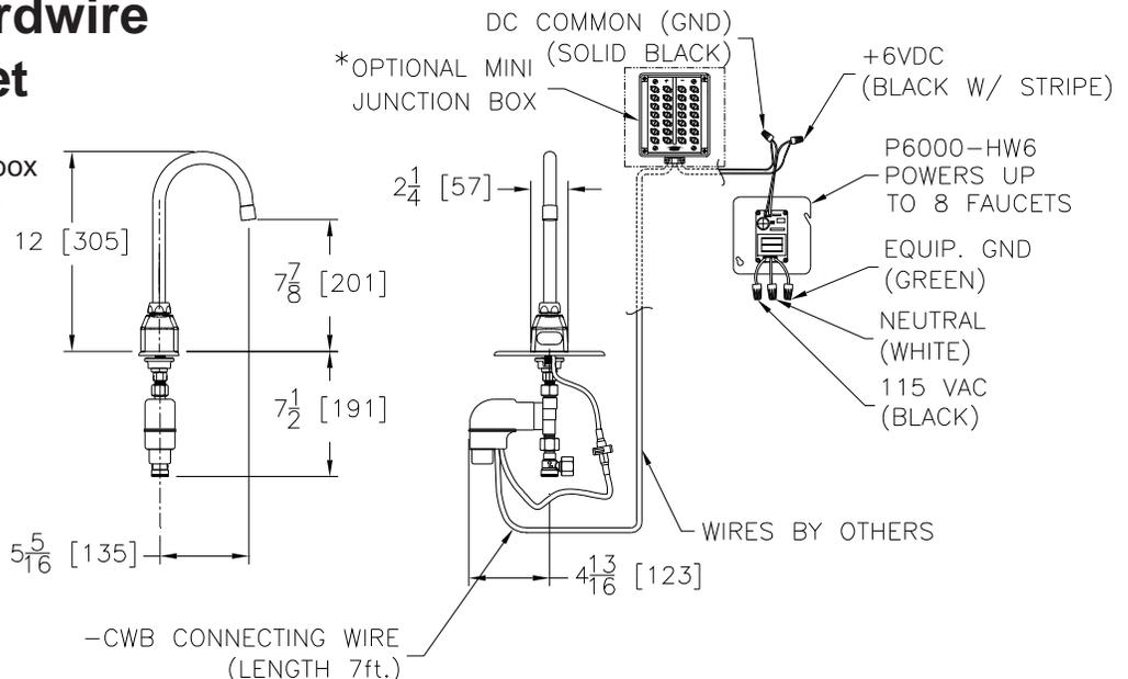
**NOTE: MUST USE EITHER ZURN P6000-HW6 HARDWIRE POWER CONVERTER OR ZURN P6900-ACA PLUG-IN POWER CONVERTER TO ENSURE PROPER OPERATION. USING A POWER CONVERTER OTHER THAN ZURN MAY RESULT IN OPERATION MALFUNCTION OR UNIT FAILURE.**
